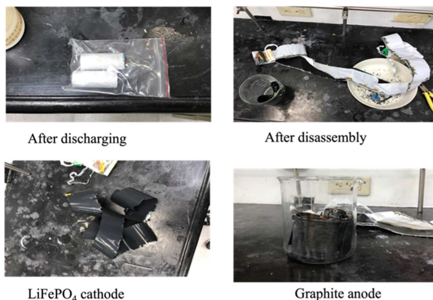
Figure 1. Positive LFP electrode separated from the negative electrode (graphite) and electrolyte.
