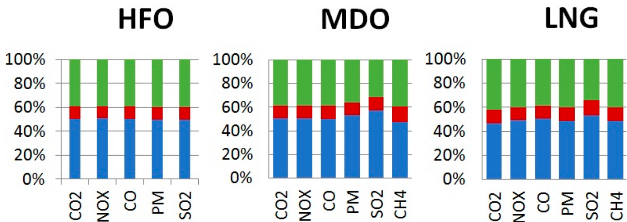
Figure 5. Total exhaust emissions during ship operational modes (cruising (blue colour)–manoeuvring (green colour)–hotelling (red colour)) per fuel type.
