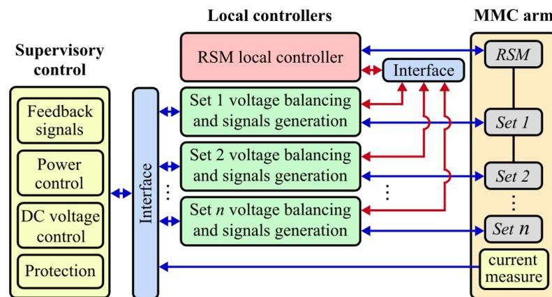
Figure 3. The proposed control structure for an MMC-arm.
