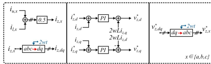
Figure 6. Circulating current suppression control diagram.
