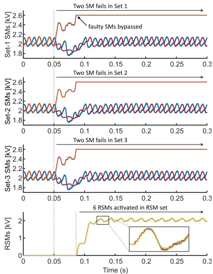
Figure 11. SM voltage results in multiple SM failures.
