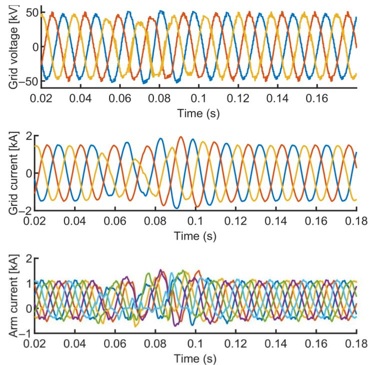
Figure 12. MMC performance results in multiple SM failures.
