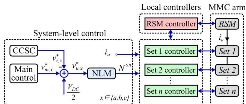
Figure 4. Overall MMC control structure.
