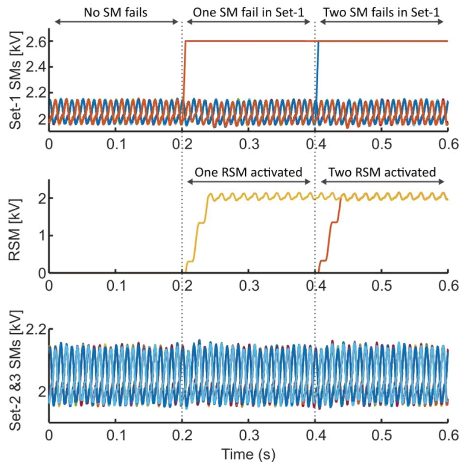
**Figure 10.** MMC SM voltage results in SM failures in set 1.
