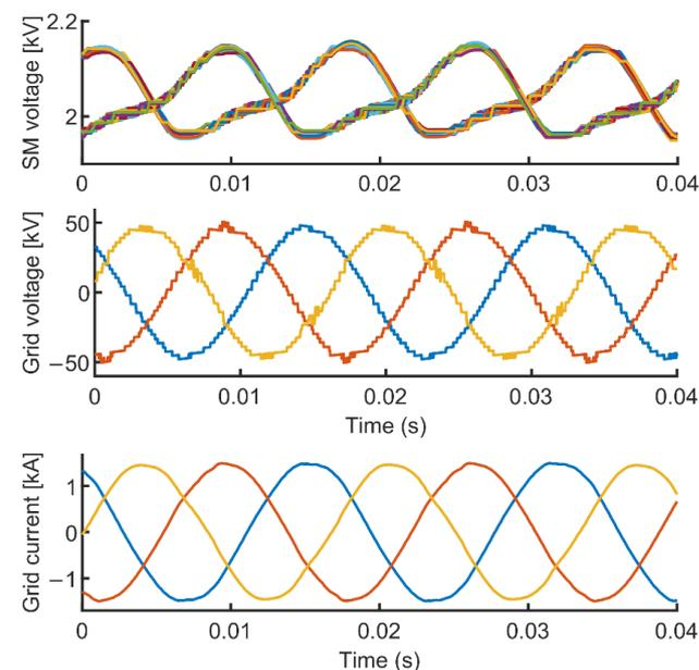
**Figure 8.** MMC performance under normal conditions (Steady State).
