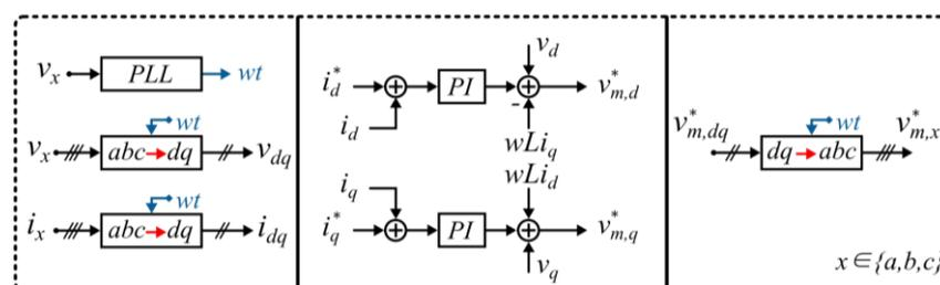
Figure 5. Main control diagram.
