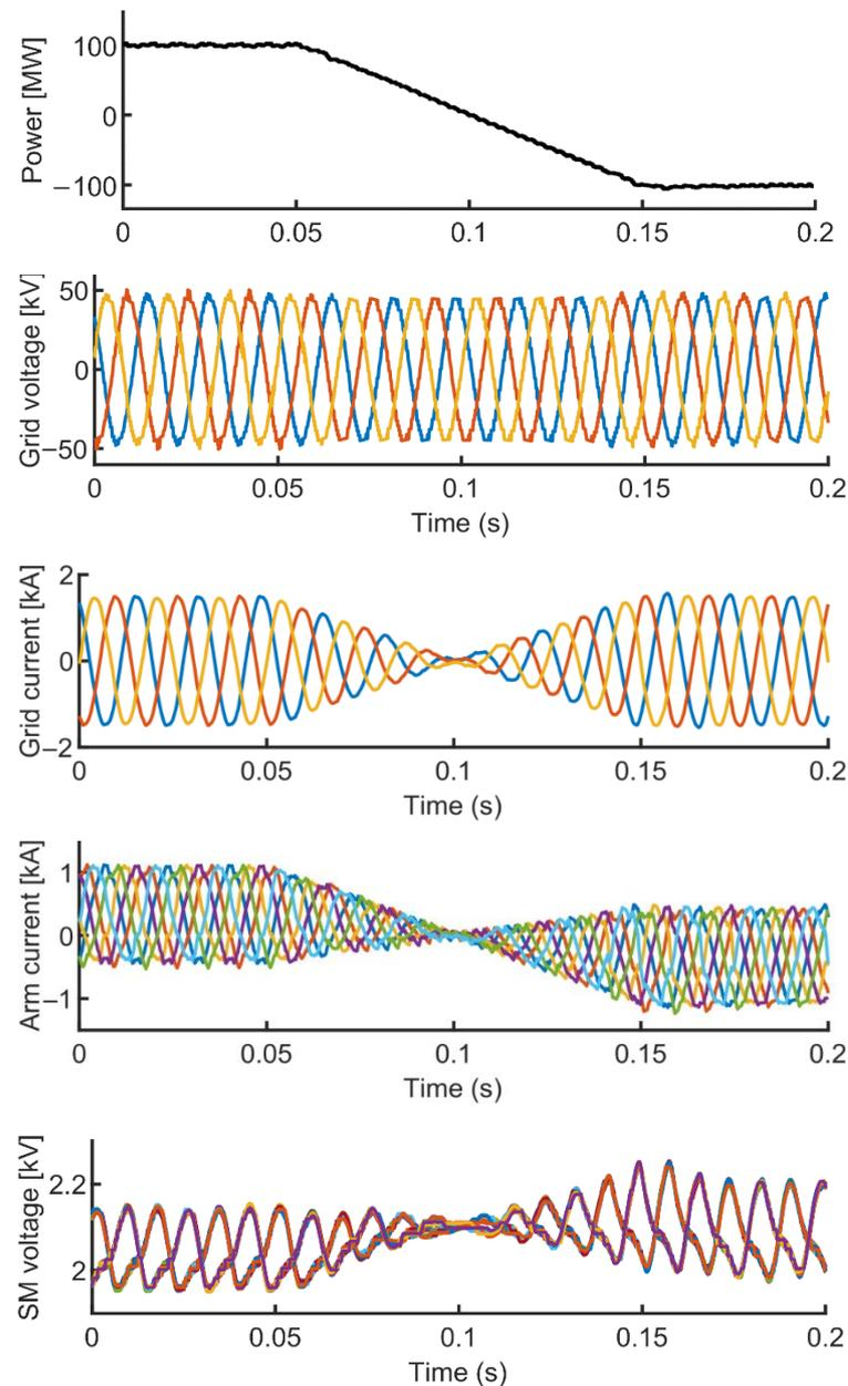
**Figure 9.** MMC results under transient conditions (power ramp).
