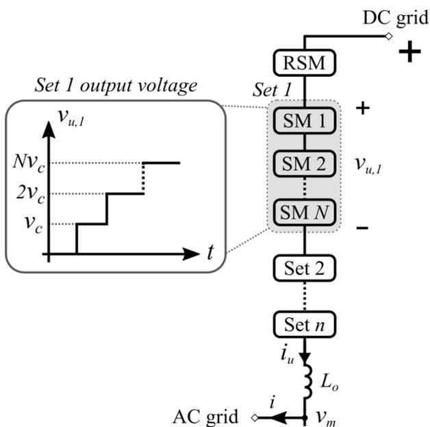
Figure 2. MMC arm operating principle.
