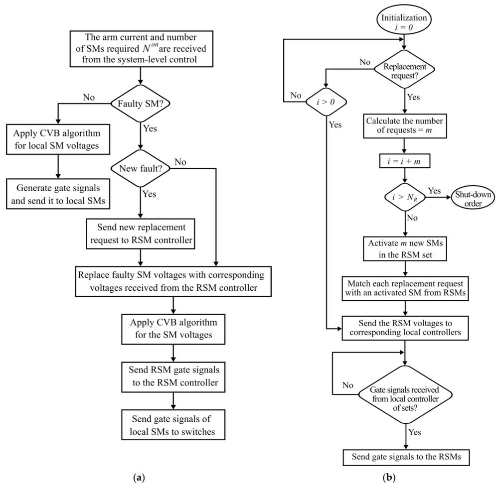
Figure 7. Controller flow chart: (a) Non-redundant local controller; (b) RSM’s controller.
