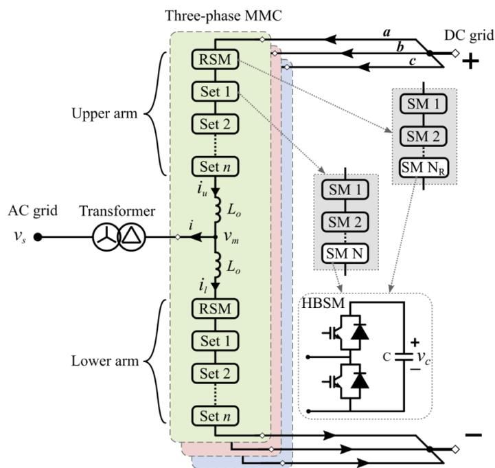
Figure 1. Three-phase MMC system.
