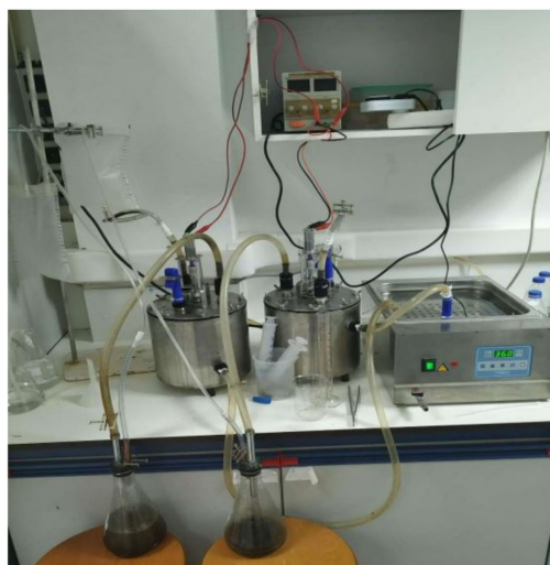
Figure 1. Experimental setup of the anaerobic digestion reactor used in this study.
