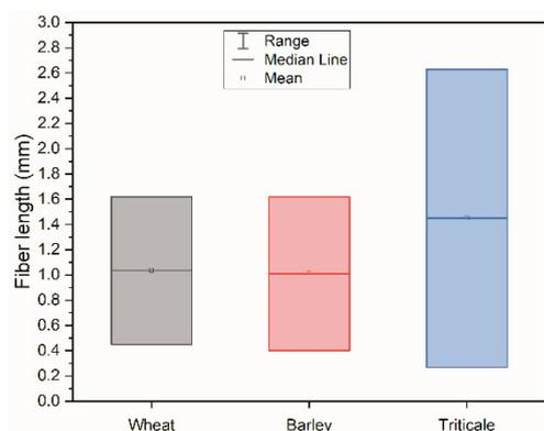
**Figure 1.** Fiber length of straw used in the production of laboratory paper.
