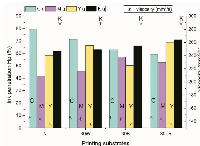
Figure 8. Ink penetration depth on gravure prints compared to the property of printing ink viscosity.
