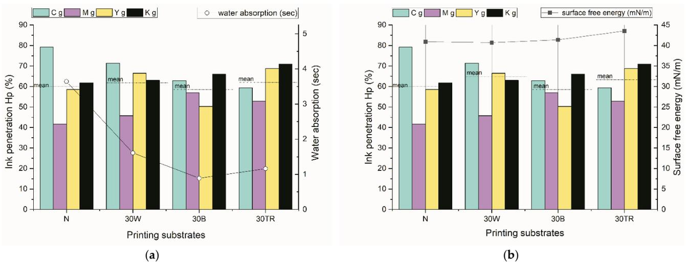
Figure 7. Ink penetration depth on gravure prints compared to the characteristics of the printing substrate: (a) water absorption and (b) surface free energy. Note: the mean penetration values of cyan, magenta, yellow and black printing inks on the same substrate are shown and labeled “mean”.
