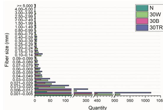
Figure 10. The quantity of fibers within each printing substrate in relation to the fiber size.
