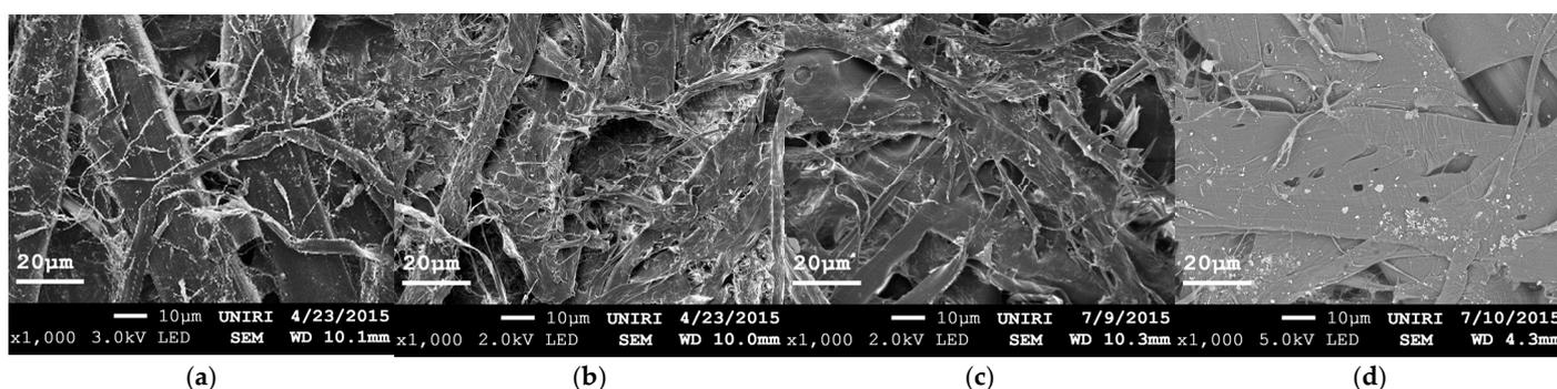
**Figure 2.** SEM images (magnification 1000×) of laboratory papers of different composition: (a) N; (b) 30W; (c) 30B; (d) 30TR.
