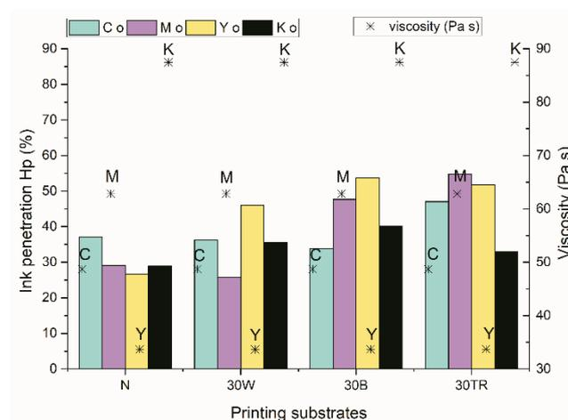
**Figure 5.** Ink penetration depth on offset prints compared to the property of printing ink viscosity.
