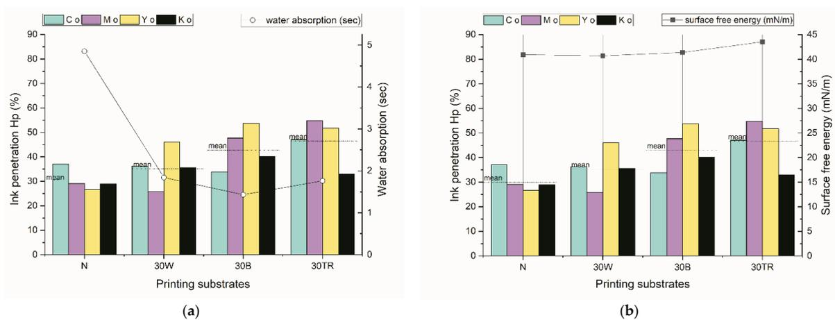
**Figure 4.** Ink penetration depth on offset prints compared to the characteristics of the printing substrate: (a) water absorption and (b) surface free energy. Note: the mean penetration values of cyan, magenta, yellow and black printing inks on the same substrate are shown and labeled “mean”.
