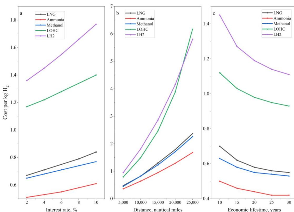
**Figure 6.** Sensitivity analysis on some selected parameters: (a) interest rate, (b) distance of the shipping route, (c) economic lifetime.
