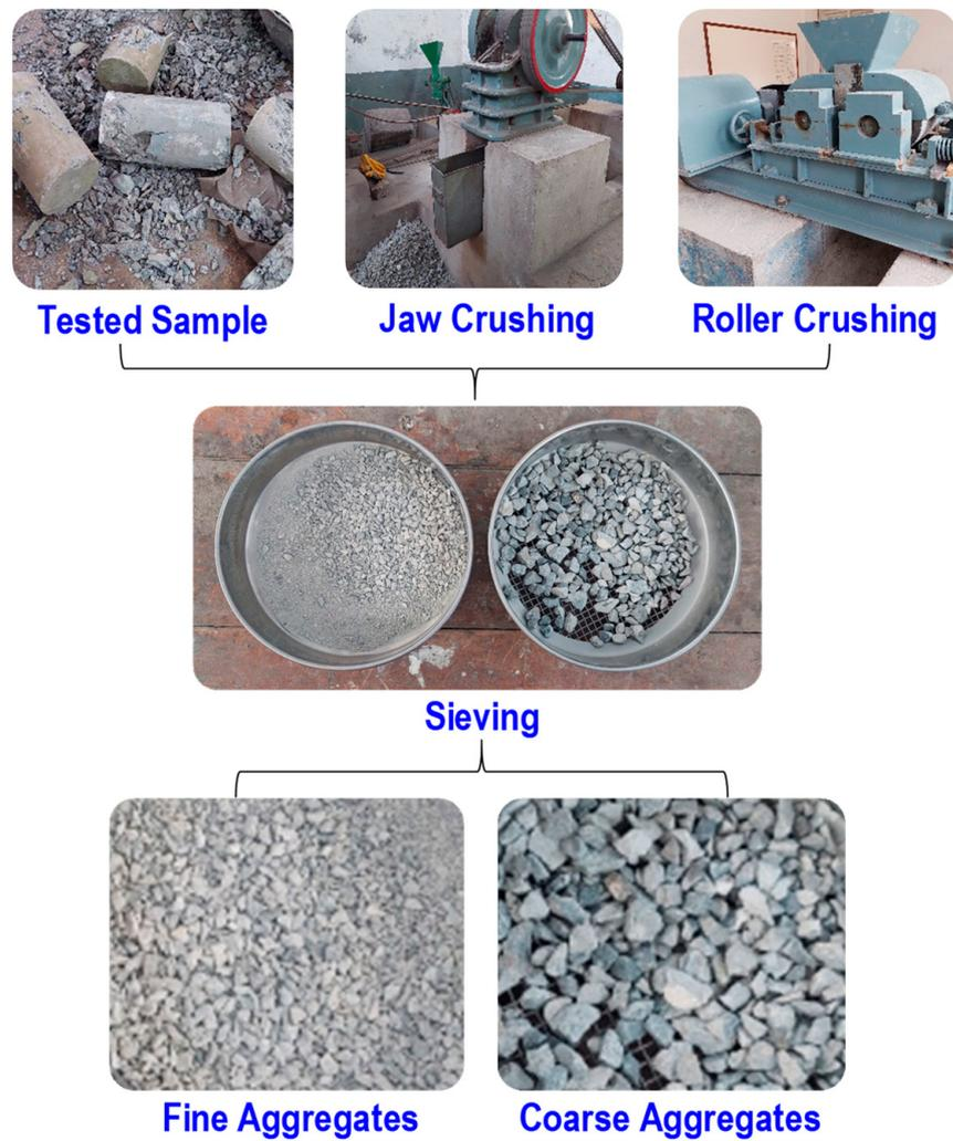
Figure 2. Process of production of recycled concrete aggregates.
