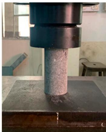
**Figure 7.** Compression test on concrete cylinder.
