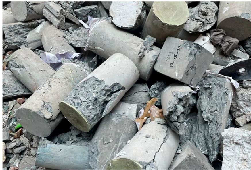
Figure 1. Crushed samples of concrete as source of RA.
