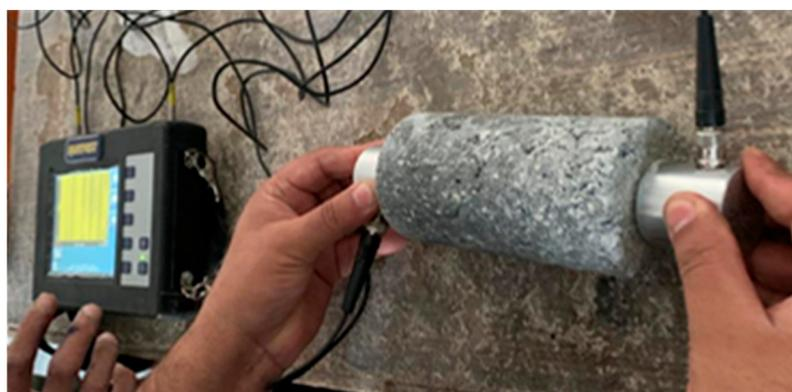
Figure 10. UPV testing device.
