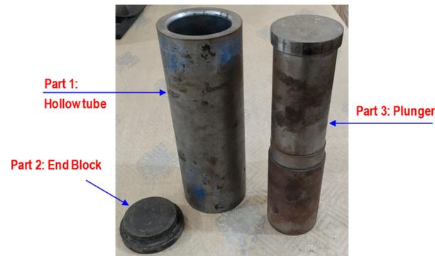
**Figure 4.** Metallic mold prepared for compression casting.
