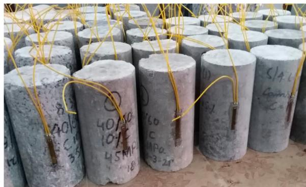
Figure 8. Samples with strain gauges pasted on their surface.
