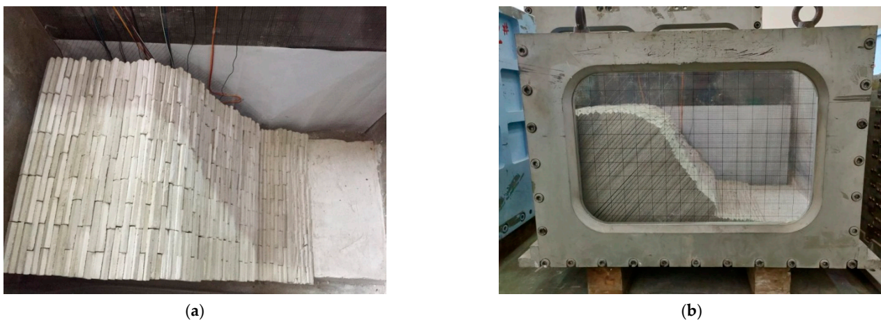
Figure 3. Model construction: (a) top view of slope model; (b) completed model in the test box.
