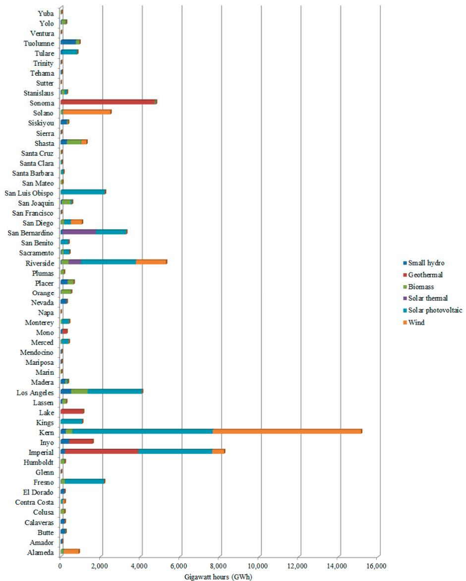
**Figure 4.** Utility-scale renewable electrical generation by county in California for each RE type in 2019. Data from the California Energy Commission [34].
