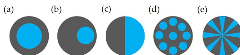
Figure 6. Different cross sections of bicomponent fibers: (a) core/sheath (concentric), (b) core/sheath (eccentric), (c), side-by-side, (d) islands-in-the-sea, and (e) Segmented pie [31]. Reprinted with permission.
