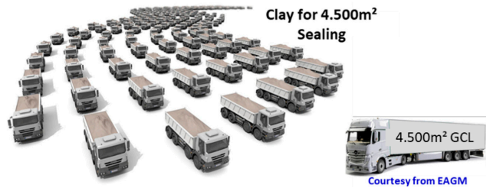
Figure 5. Illustration of fewer truckloads required for a site when geosynthetic materials are used, compared to the traditional solution.
