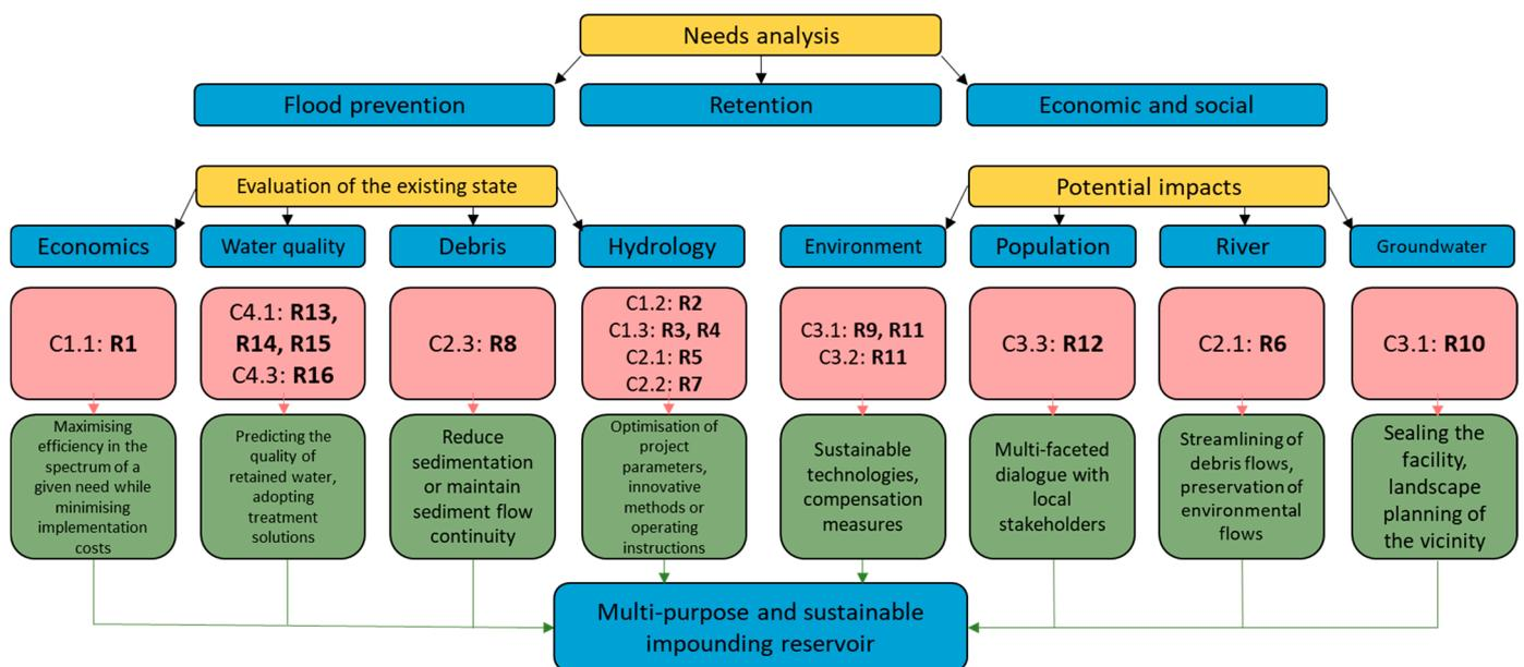
Figure 7. The most important issues to be considered during the planning and construction of reservoirs.
