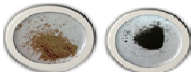
Figure 1. Picture of graphitic carbon nitride before and after doping with bimetallic silver and copper (Ag-Cu).
