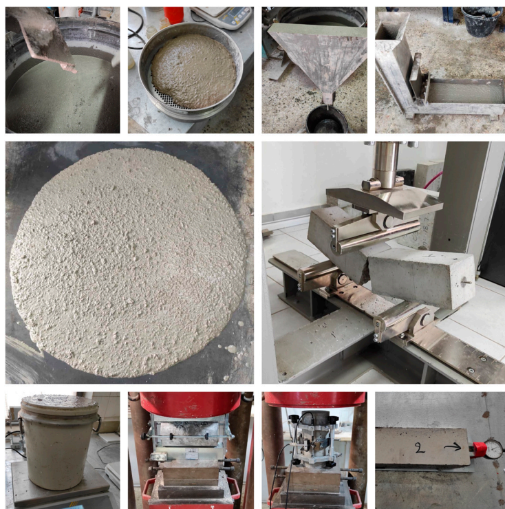
Figure 4. Indicative photos of the experimental procedures for fresh and hardened SCC mixtures produced.
