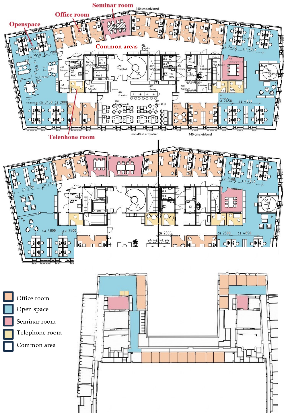
Figure 2. Floor plans of Department A (2 floors, top two floor plans) and Department B (bottom floor plan). Orange: office rooms. Blue: open spaces. Red: seminar rooms. Yellow: telephone rooms. White: Common areas such as corridors, kitchen, and toilets.
