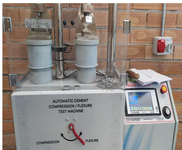
Figure 8. Compressive and flexural strength test machine.
