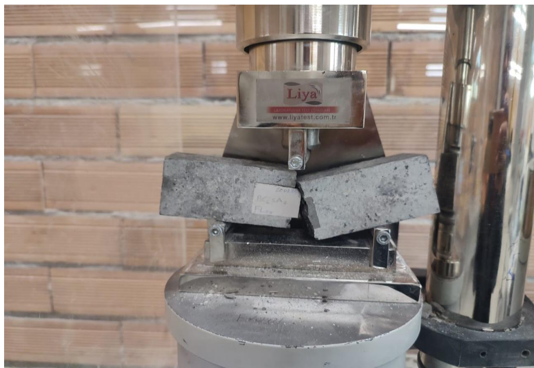
Figure 9. Flexural strength testing.
