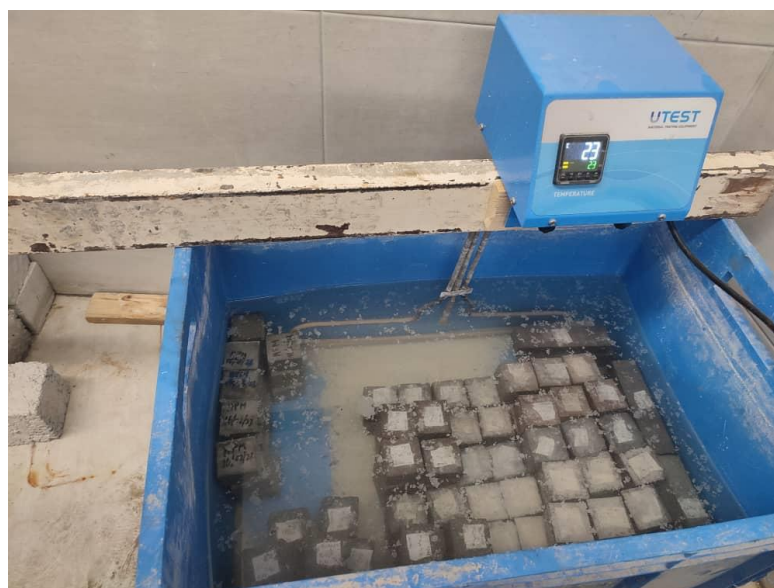
Figure 6. The sample curing process.
