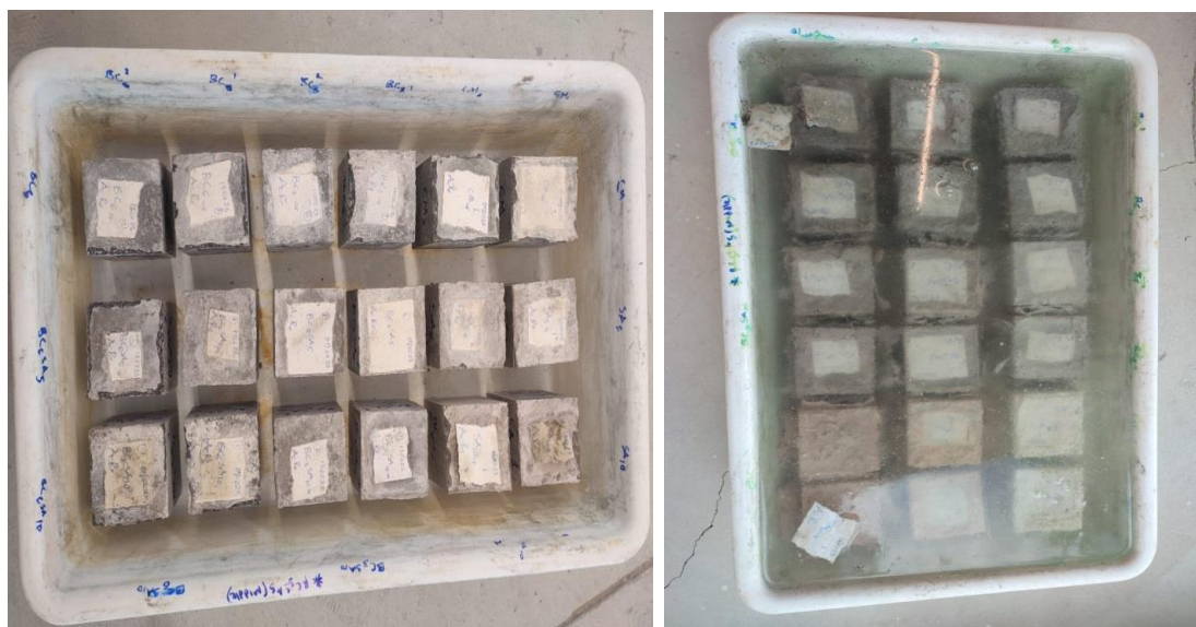
Figure 21. The samples exposed to sulfuric acid.
