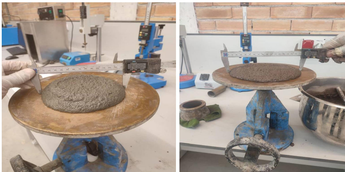
Figure 7. Flow table test.
