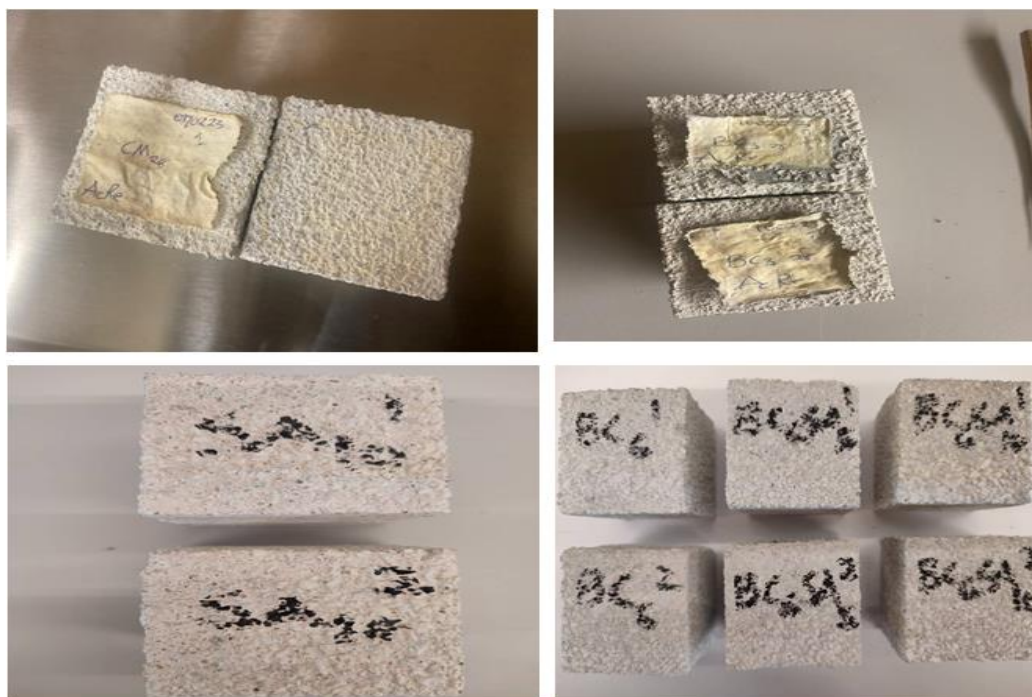
Figure 22. Surface degradation of all mixtures after sulfuric acid attack.
