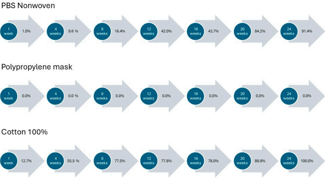
Figure 10. Results of biodegradation process of PBS nonwoven, polypropylene mask and cotton 100%.
