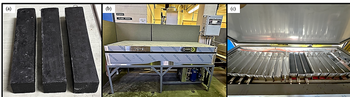
Figure 8. Freeze–thaw test setup for stone veneer samples: (a) cylindrical samples, (b) automatic rapid freeze–thaw testing machine, and (c) samples placed inside the freeze–thaw testing machine.
