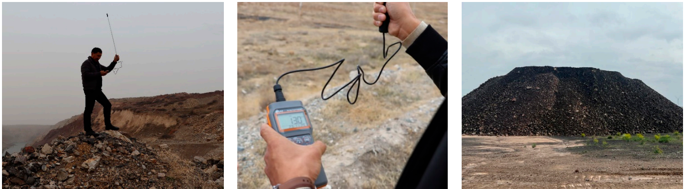
Figure 2. Wind speed measurements in the area of ore dumps in Zhanatas (photos by D. Aliaskarov, Sh. Laiskhanov).
