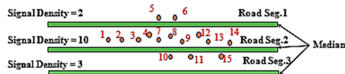
Figure 2. Illustration of signal confusion among lanes: there is a vehicle running on lane 2 (road segment 2), with 15 GPS signals received during the movement. Due to GPS signal transmission errors and small lanes, some confusion occurred; signals 5 and 6 were mistaken for lane 1 (road segment 1), and signals 10, 11, and 15 were mistaken for lane 3 (road segment 3).
