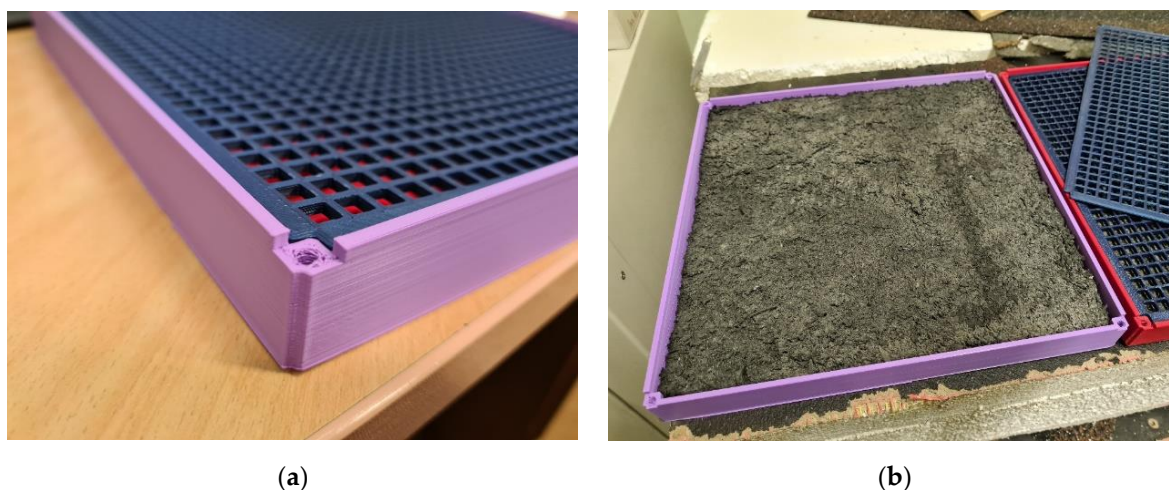
Figure 3. Perforated cartridges for installing the rubber granulate plate. (a) The 3D-printed cartridge without the rubber granules; (b) the 3D-printed cartridge filled with the rubber granulate.
