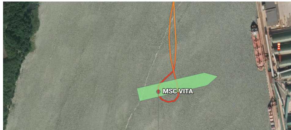
Figure 6. Trajectory of the POST PANAMAX container vessel during turning in the port ship turning basin ( T/H about 0.95) received by the calibrated simulator and on the real ship.
