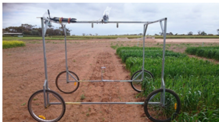
Figure 1. The platform used to capture images of plants in the field. The manually propelled platform is comprised of a custom-built steel frame and four bicycle tyres. A colour chart for calibration and up to five cameras can be mounted on it (stereo top view, stereo oblique view, and one side view).
