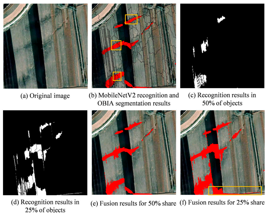
Figure 13. OBIA and MobileNetV2 recognition results and segmentation data fusion (the 50% share area is displayed in the figure's box).
