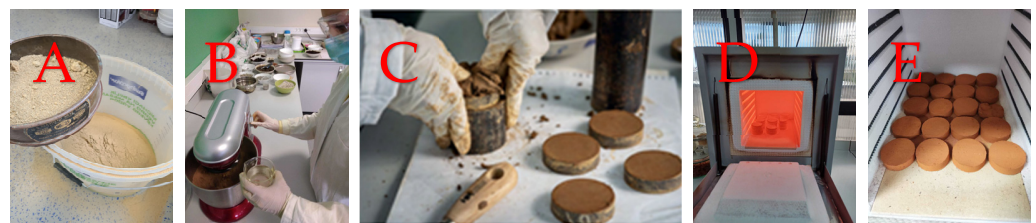
Figure 1. Production of modified laboratory bricks with different mass proportions of EMS (A) Sieved through sieve, (B) Homogenisation of solid raw materials, (C) Pressed into moulds, (D) Heat treatment in an annealing furnace and (E) Modified bricks.
