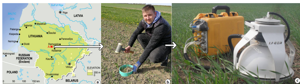
Figure 1. The investigation soil CO 2 efflux ((a)—long-term field experiment site (A); (b)—preparation for CO 2 measurement; (c)—measurement of CO 2 efflux by LI-COR 8100A).
