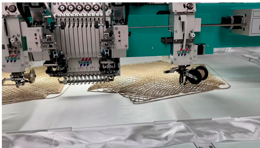
Figure 3. Tailored Fiber Placement (TFP) of flax fibers. ©BioMat.
