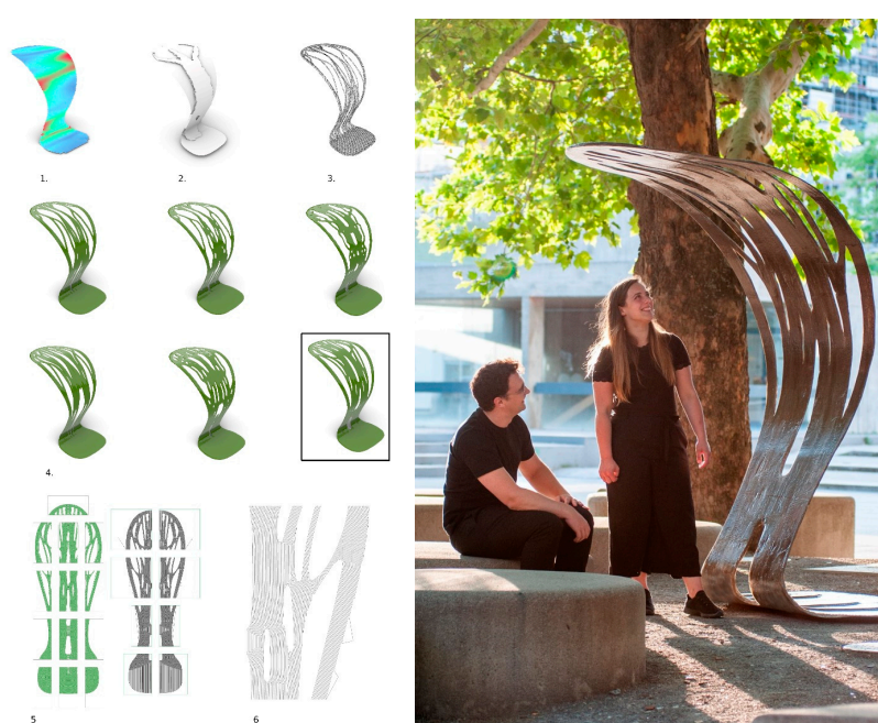
Figure 4. (Left): Design process: (1) basic shell optimization, (2) topology optimization of a single-curved canopy, (3) generated structure by agents attracted by results from topology optimization,
