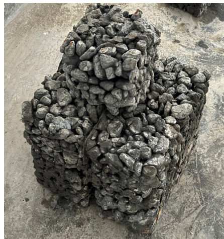
Figure 1. Plant-growing ecological concrete.
