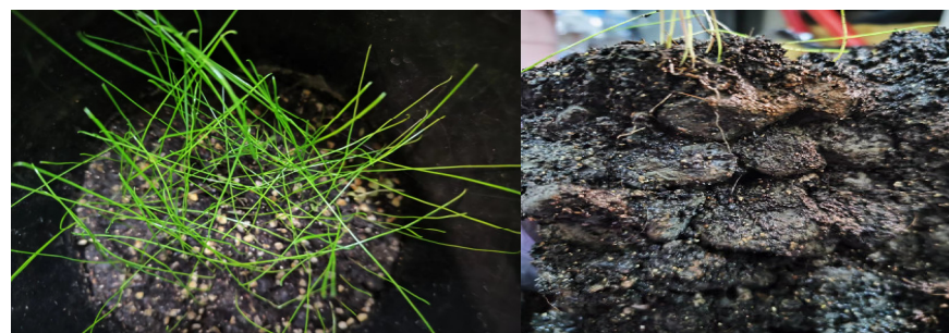
Figure 7. Vegetation performance of ecological concrete.
