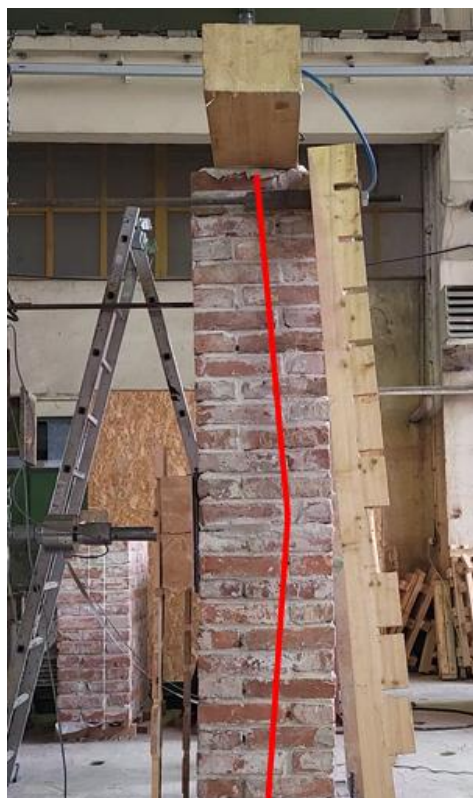
Figure 11. Vertical bending failure mechanism.
