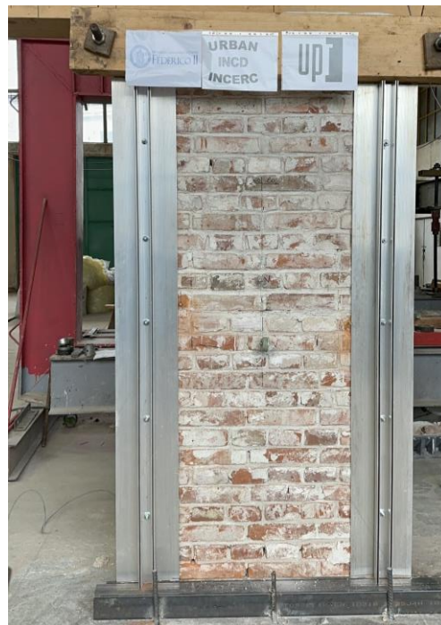
Figure 14. Masonry wall reinforced with aluminium profiles.
