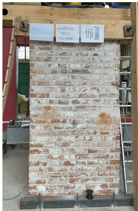
Figure 3. The masonry wall obtained from the union of two panels.
