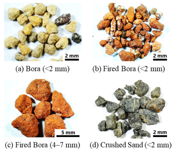
Figure 1. Microscopic images of un-fired and fired Bora samples and crushed sand.
