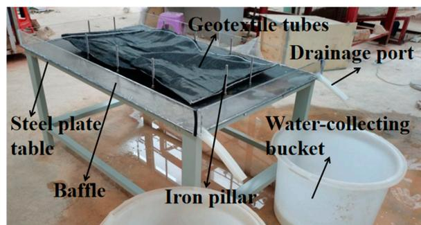
**Figure 2.** Geotextile tube-filling and consolidation test setup.
