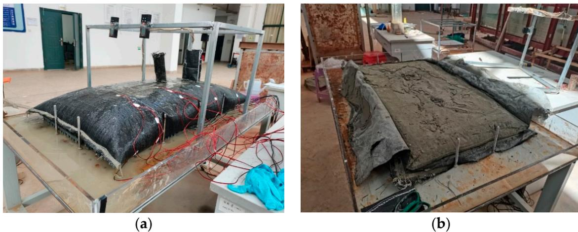
**Figure 4.** Diagram of drainage and consolidation process of geotextile tubes. (a) Geotextile tubes drainage. (b) Geotextile tubes consolidation.
