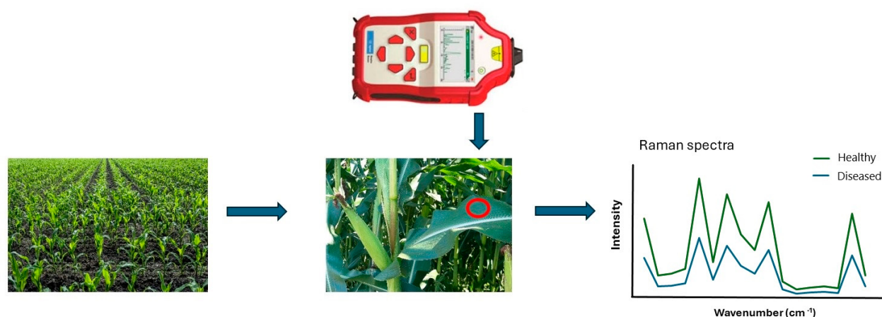
Figure 4. Scheme of using portable Raman spectroscopy to assess the health of crop plants.
