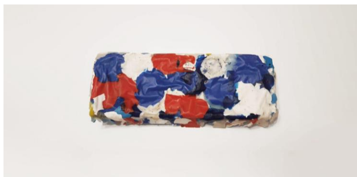
Figure 4. A sample product from hard-to-recycle plastics formed in a steel mold.
