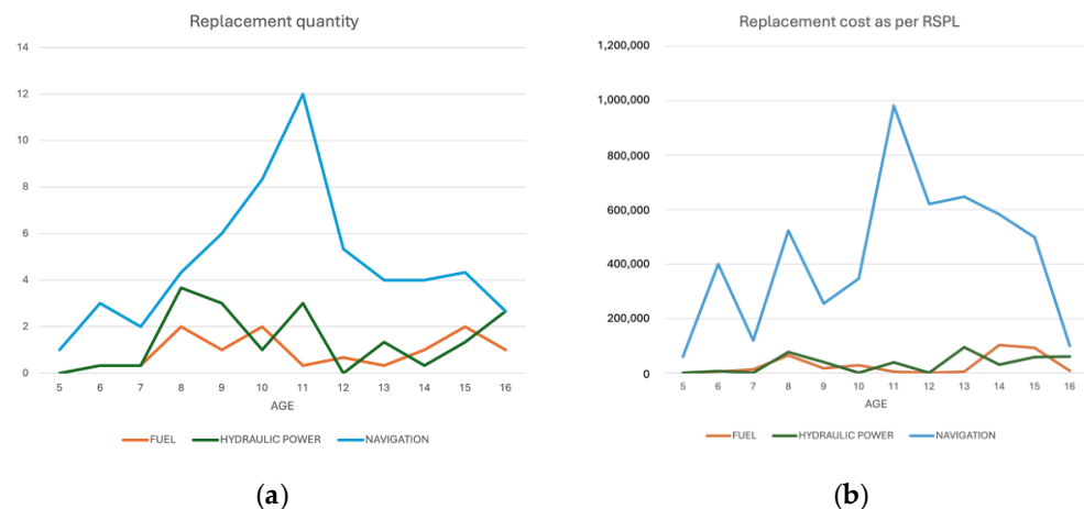
Figure 5. Replacement quantity of different aircraft systems (a) and the corresponding replacement costs for these systems (b) over the age of the aircraft.
