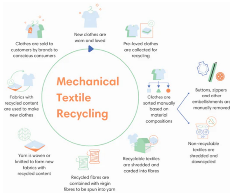
Figure 9. Overview of mechanical recycling of textiles. Reproduced with permission from: https://tortoisethelabel.com/blogs/journal/types-of-textile-recycling , accessed on 11 July 2024. Copyright: Tortoise the Label Private Limited.
