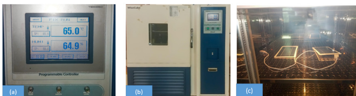
Figure 9. (a) shows panels subjected to 65 °C and 65% RH. (b) Temperature and humidity chamber placed in lab. (c) shows inside view of solar panels placed under damp heat conditions.
