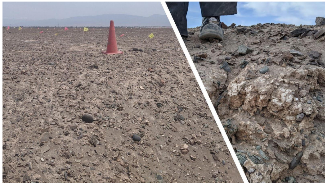
Figure 4. Geophysical testbed established atop the future Majes II agricultural site. A shallow erosional channel exposing caliche deposits was located immediately outside of the 30 m × 40 m survey grid (photographs taken by R. Krahenbuhl).
