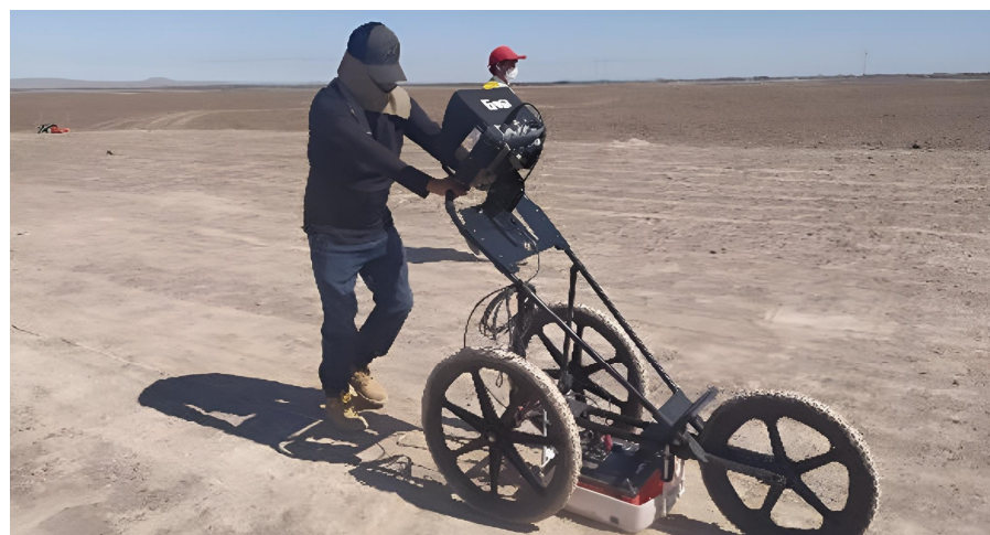
Figure 6. Ground penetrating radar (GPR) data being acquired above the caliche testbed using the GSSI system.
