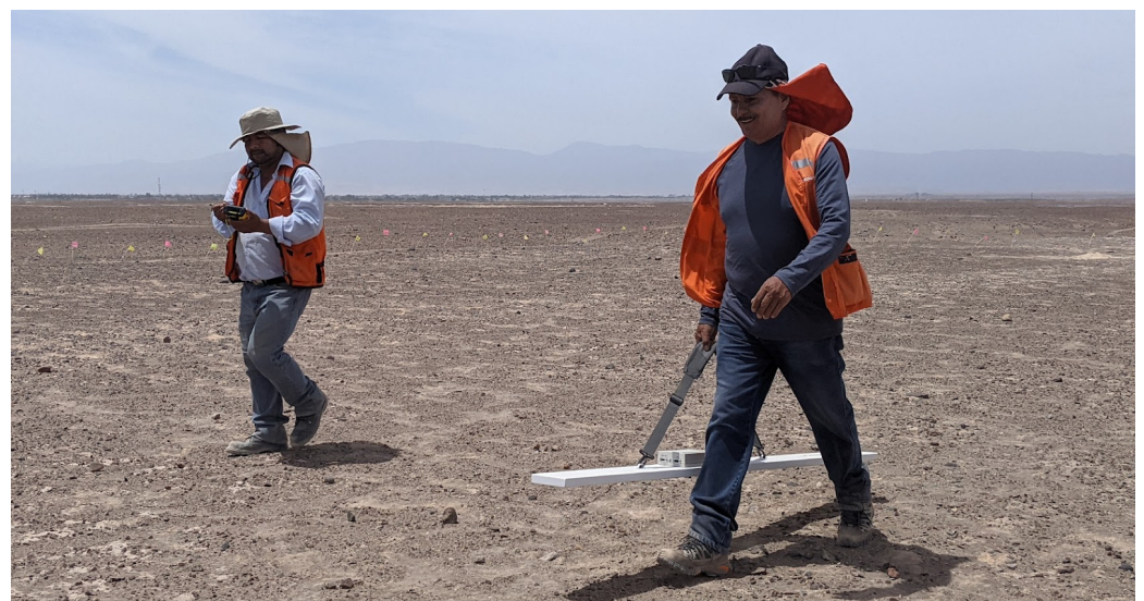
Figure 5. GEM-2 FDEM survey above the caliche testbed at Majes II (photo by R. Krahenbuhl).
