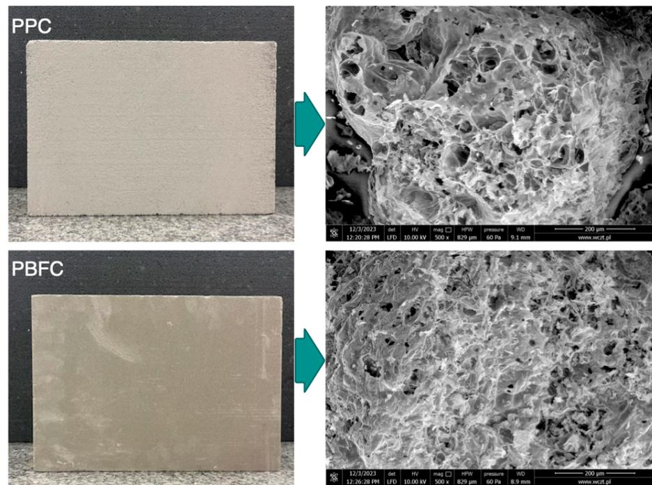
**Figure 1.** Overview photos of the two types of base perlite concrete materials used in the study: (PPC) with the addition of CEM I 52.5R cement and (PBFC) with the addition of CEM III 42.5R cement.
