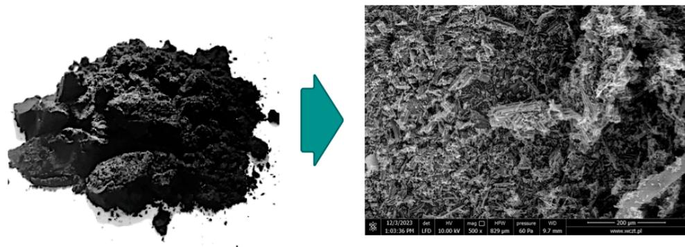
**Figure 3.** Overview photo of the activated carbon used in the study and SEM image of its structure at approximately  $200 \mu\text{m}$ .
