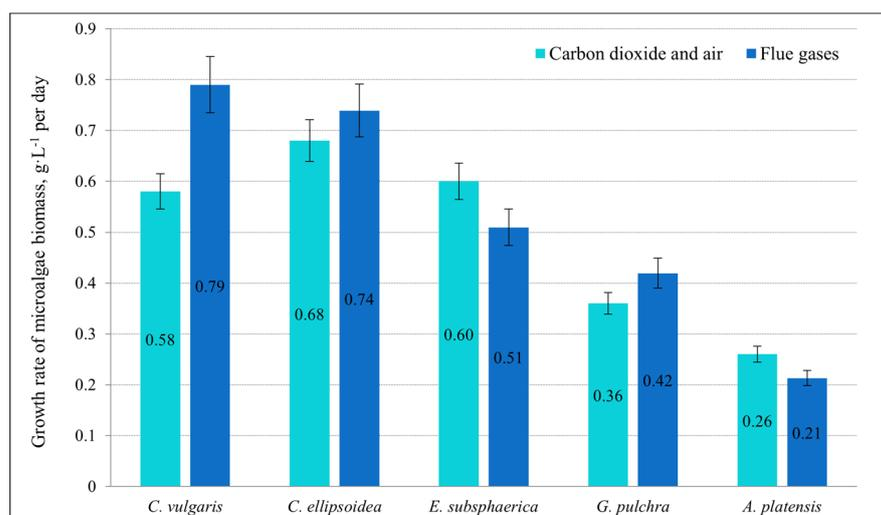
**Figure 3.** The growth rate of microalgae biomass ( $\text{g}\cdot\text{L}^{-1}\cdot\text{d}^{-1}$ ) in the experiments with carbon dioxide and air (from our previous article [36]) and flue gas (this work).  $\text{CO}_2 = 6\%$  and illumination  $200 \mu\text{mol quanta}\cdot\text{m}^{-2}\cdot\text{s}^{-1}$ . The error bars represent standard deviation.
