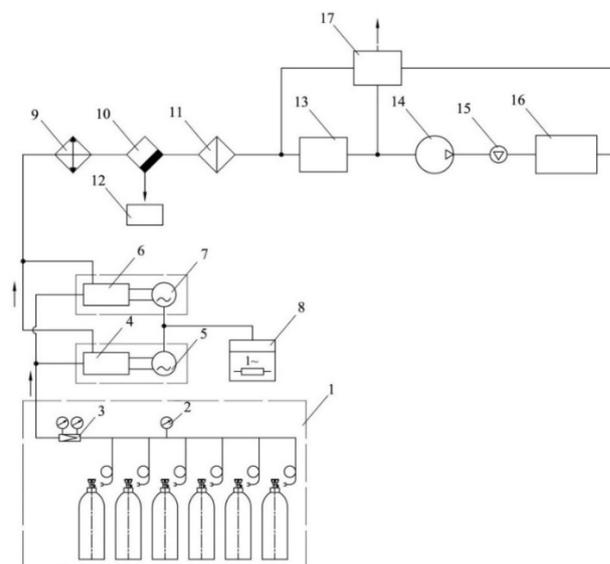
**Figure 2.** The scheme of FGGP. 1—methane discharge ramp, 2—manometer, 3—gas reducer, 4,6—internal combustion engine, 5,7—generator, 8—heater, 9—cooler, 10—condensate collector, 11—filter, 12—condensate container, 13—mixing device, 14—compressor, 15—rotameter, 16—photobioreactor, 17—buffer container.
