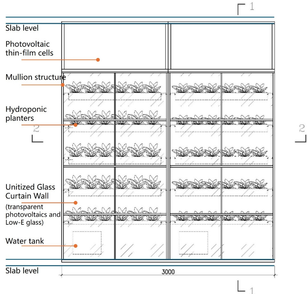
Figure 5. Technical elevation drawing of a standard ABE panel unit, detailing dimensional specifications and the spatial relationship between photovoltaic and agricultural components. The drawing includes critical measurements and component identification for fabrication purposes.
