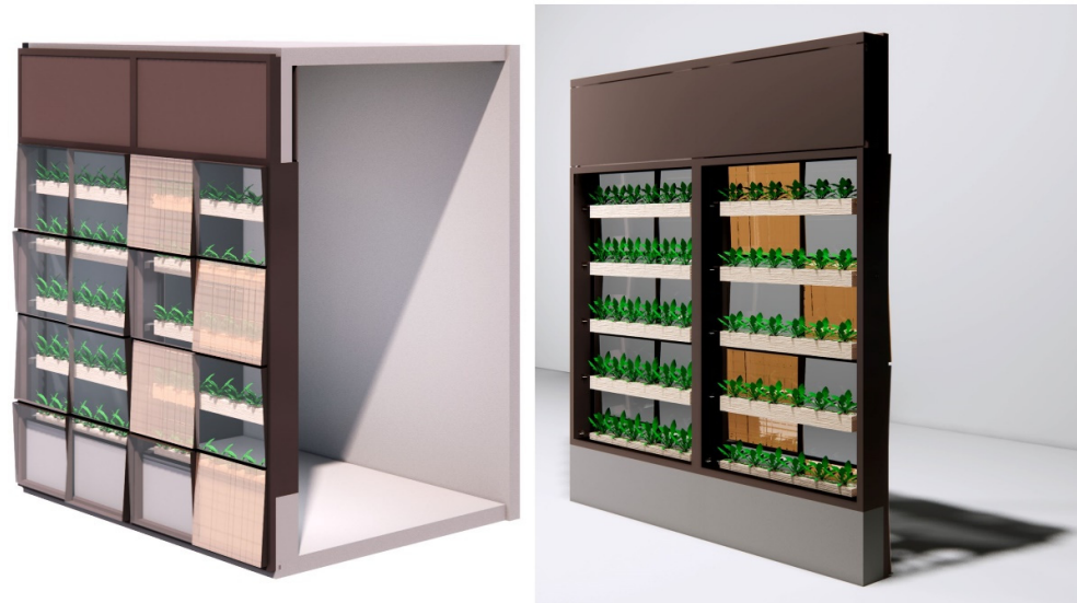
Figure 1. Overview of the agrivoltaics building envelope prototype. The (left) panel shows the front view, featuring the integrated photovoltaic panels and vertical farming modules arranged in a checkerboard pattern. The (right) panel displays the rear view, revealing the hydroponic system integration and structural support framework.
