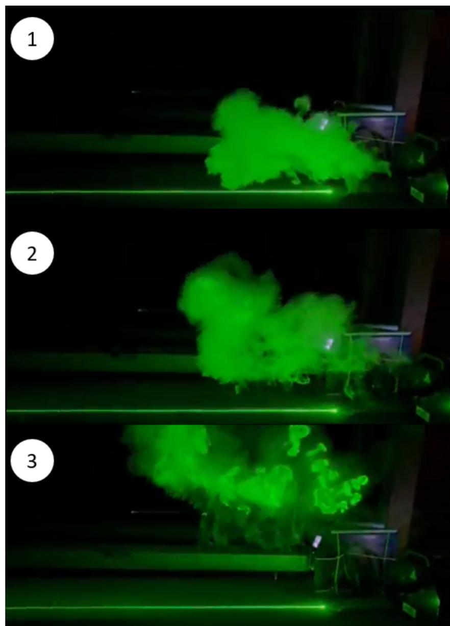
Figure 7. First Interior Rick Smoke Test.
