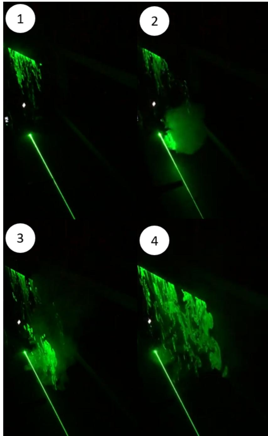
**Figure 8.** Second Interior Rick Smoke Test.
