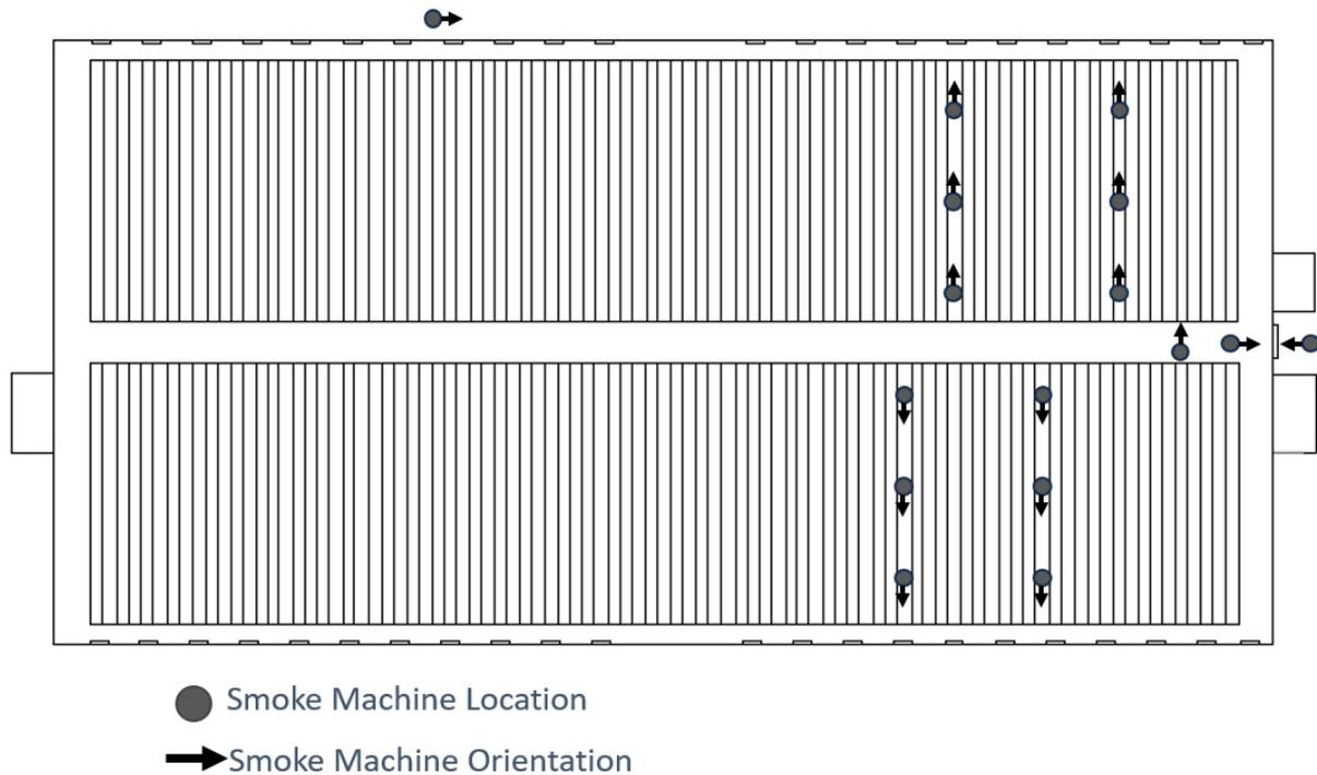
**Figure 3.** Smoke Tracing Locations.
