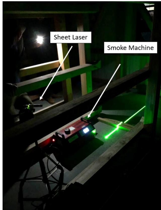
**Figure 2.** Smoke Tracing Experimental Setup.
