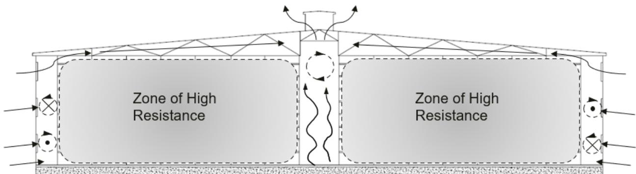
**Figure 10.** Rickhouse Section View Airflow Patterns.
