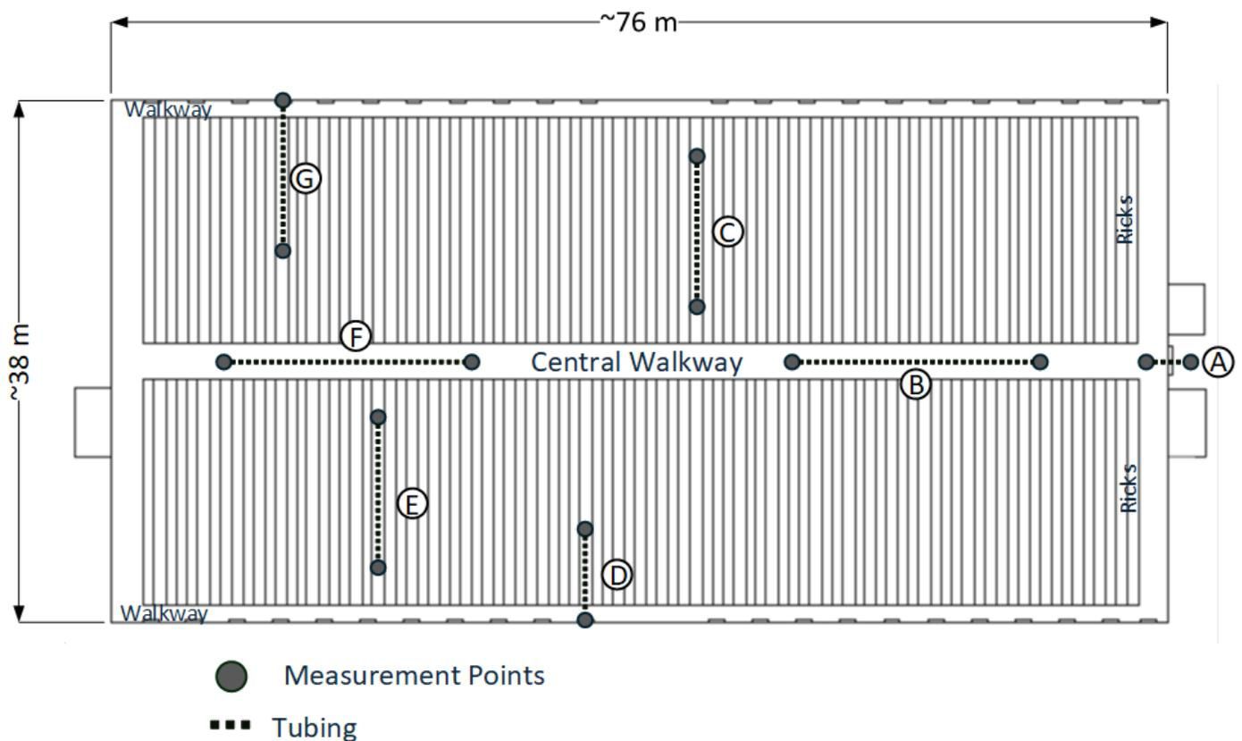
**Figure 1.** Differential Pressure Measurement Locations.
