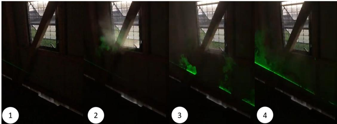
Figure 5. Windows and Ground Vent Smoke Test.
