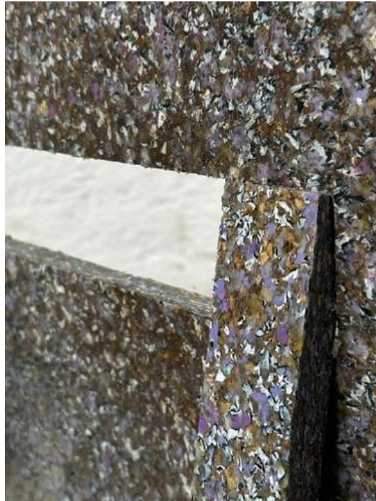
Figure 16. Laser cutting test conducted on a sample panel (ph by Design Differente).
