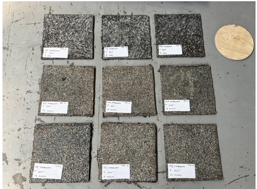
Figure 13. Subsequent tests carried out to develop the material with increased thicknesses (24 and 30 mm), aimed at verifying its stability and workability at a larger scale (ph by Design Differente).
