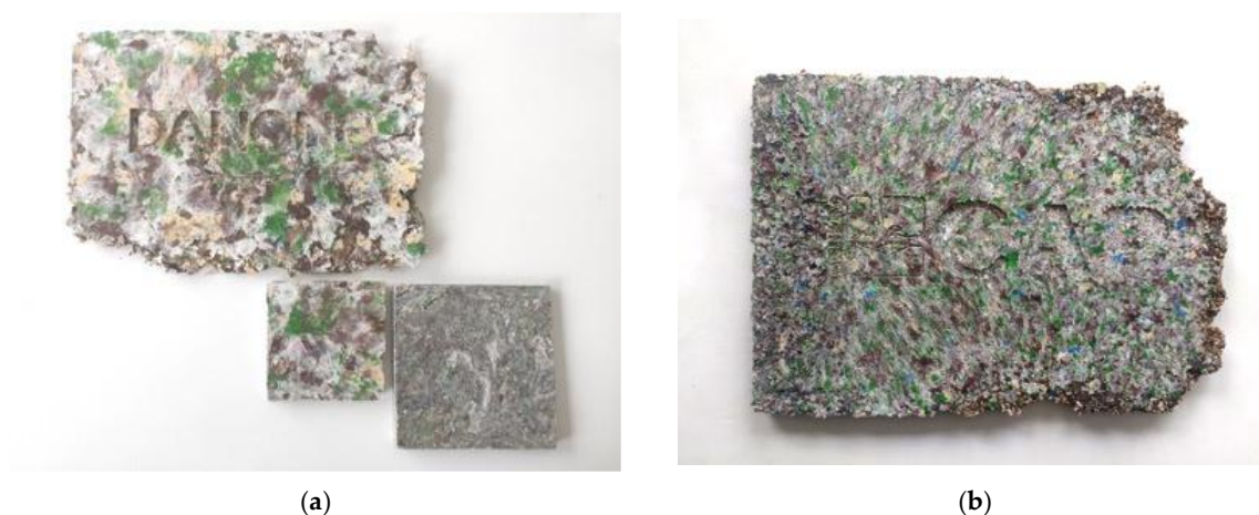
Figure 8. (a,b). Initial outcomes of the thermomechanical recycling process applied to material supplied by Gruppo CAP, using die-casting technology (ph. by Design Differente).
