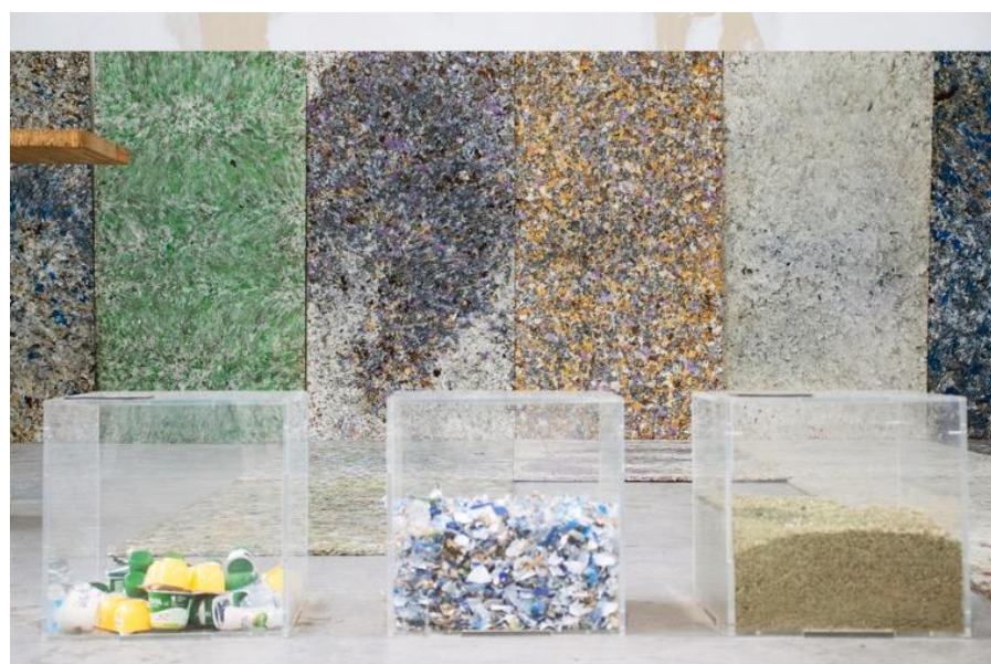
Figure 15. Colour variations of Marble CAP panels, derived from the different consumption of food products (ph. by Design Differente).
