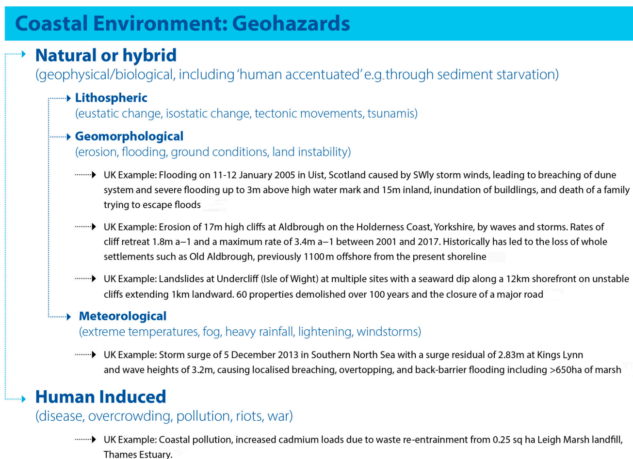
Figure 1. Conceptualisation of UK Coastal Geo-hazards. Draws on Pettit and Potts [8], data on flooding [9,10], erosion [11], landslides [12], storm surge [13], and coastal pollution [7]. Interactions between hazards are also relevant [14].
