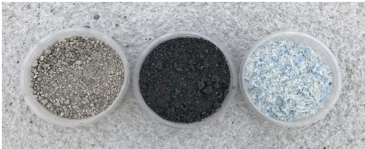
Figure 1. The materials used in the study, from right to left, are pumice, bottom ash, and PET.
