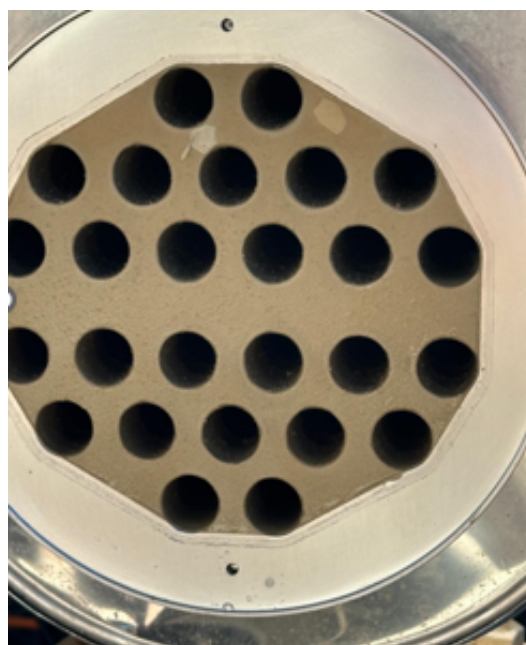
Figure 10. Salt and organic matter precipitation in MVC heat exchanger.
