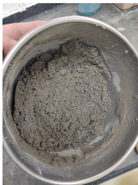
Figure 12. The cohesionless mortar mixture due to 50% of ABD replacement.
