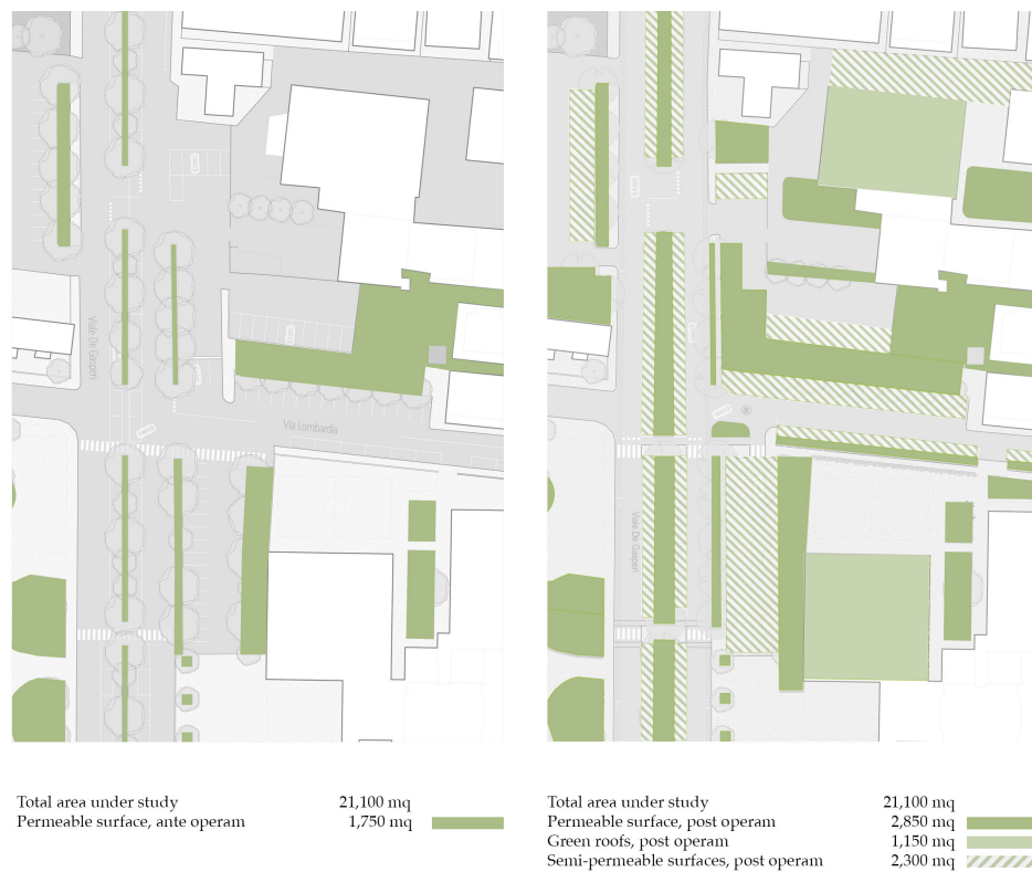
Figure 8. Plans ante operam and post operam, highlighting permeable surfaces. There is a 194% increase in permeable soil (permeable + semi-permeable soil).
