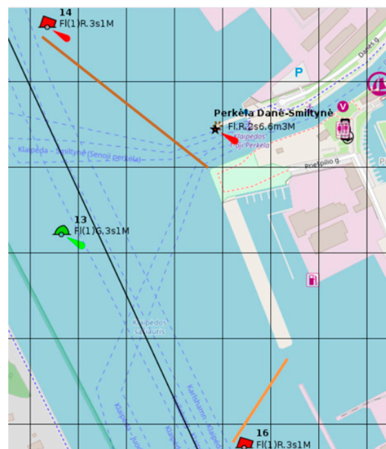
Figure 3. Dredged water area near the embankment (quay) (delimited from the embankment to the navigation channel by yellow lines).
