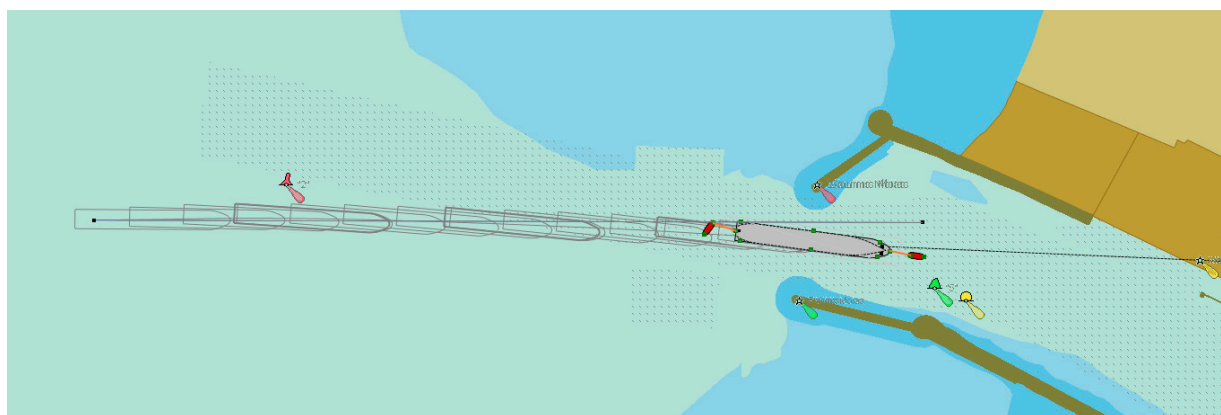
Figure 4. NEW PANAMAX container ship navigation through the port entrance channel during the vessel's entry into the port [53].
