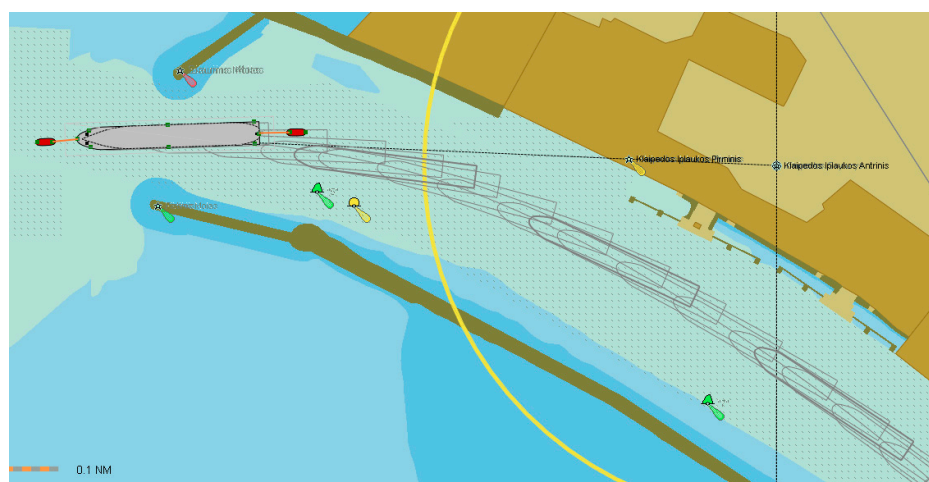
Figure 8. NEW PANAMAX container ship navigation in the inner port navigation channel and turning before approaching the port gate, when the vessel leaves the port (yellow line show light-house sector) [53].
