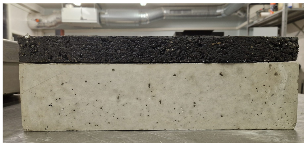
Figure 2. Specimen prepared for rolling resistance (energy loss) test.
