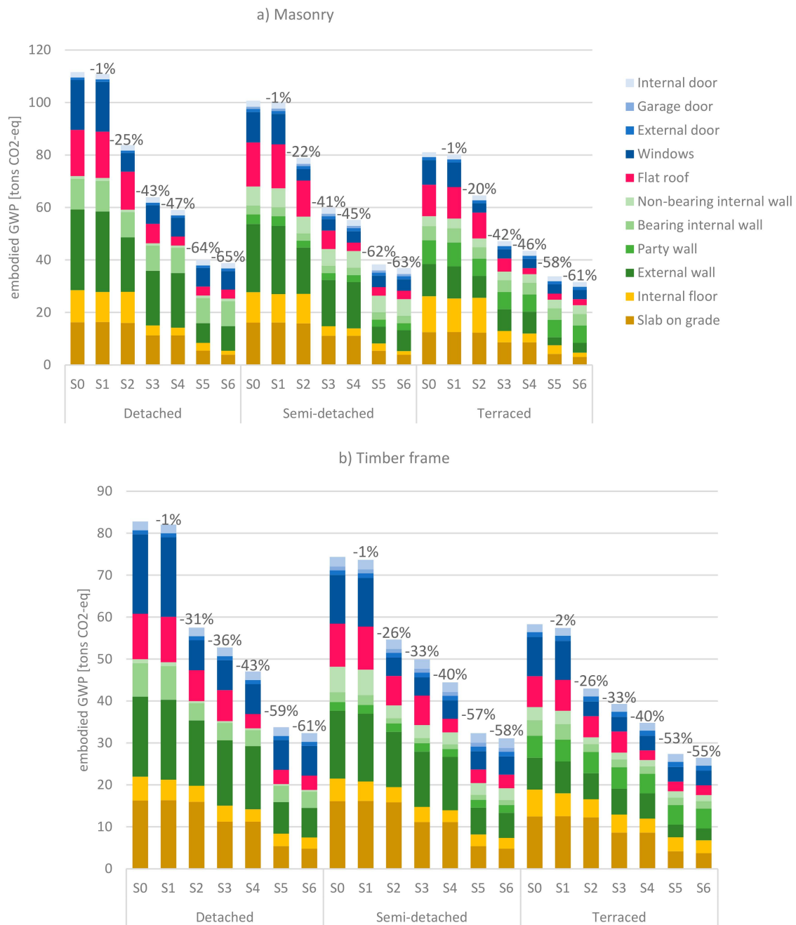
Figure A9. Stepwise reduction potential of absolute GWP for (a) masonry and (b) timber-frame construction.
